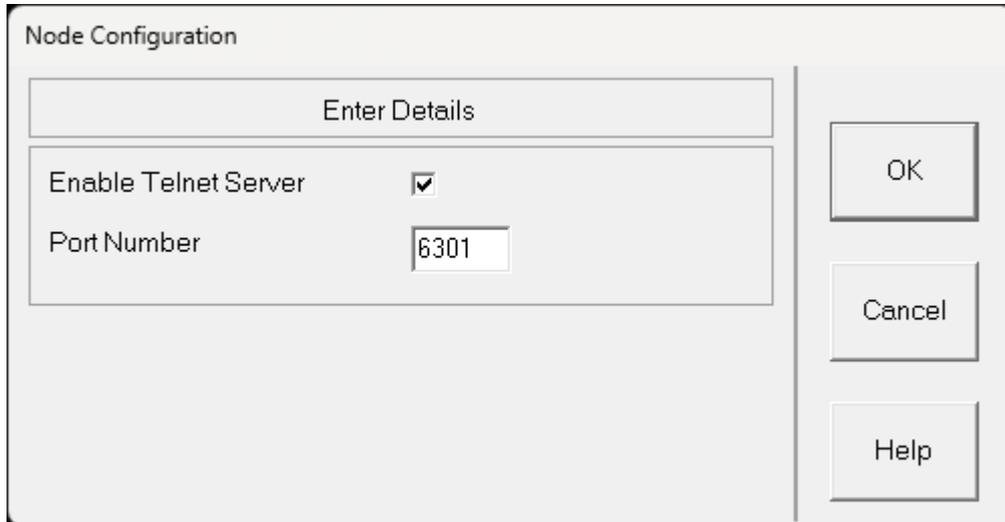
Click the tick box to enable the server and enter the desired port number.
