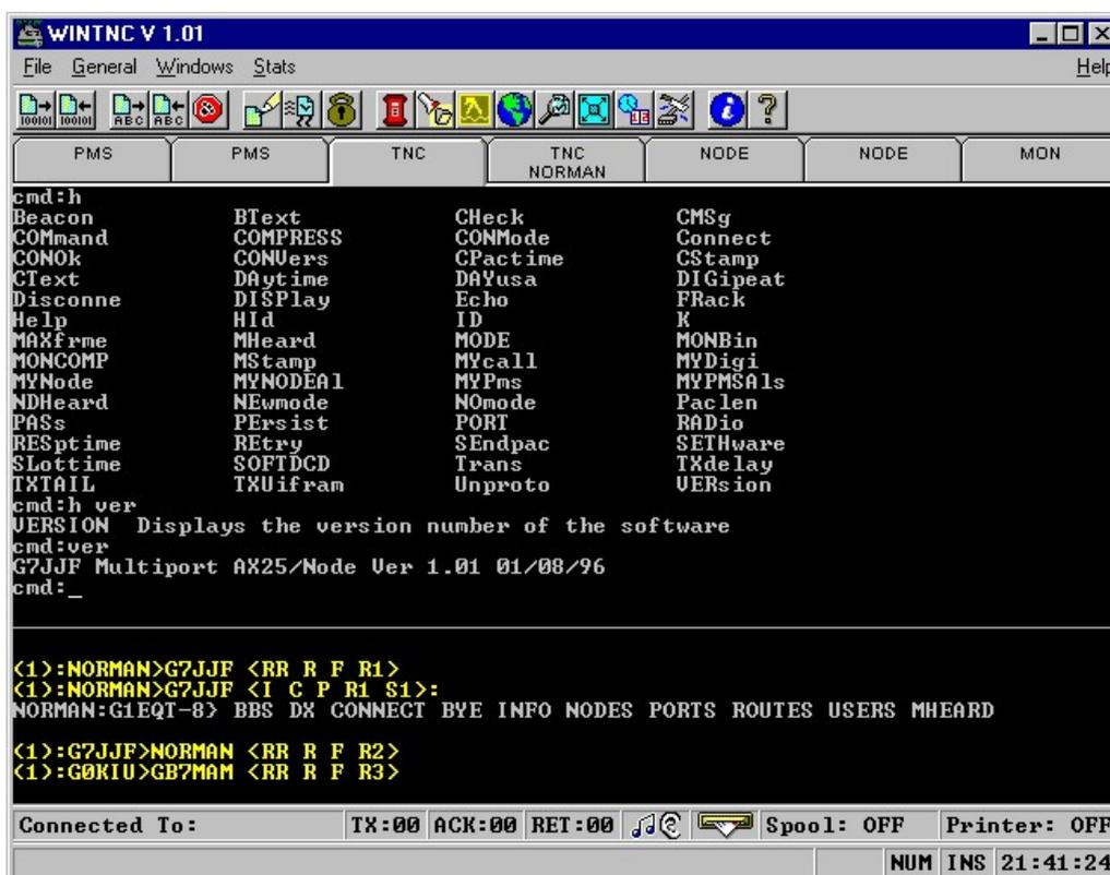
As you can see, running the software puts you into a terminal driver window. To monitor what is happening on another channel or to select a different terminal driver to use, simply click on the tab strip at the top of the screen. The tab strip shows what type each channel is together with who is currently connected to it (if anyone).
